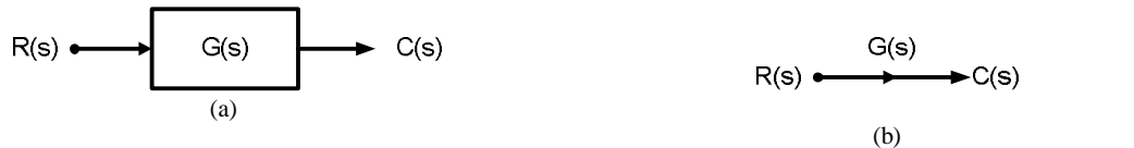
Fig.7.1. (a) Block diagram of a non-feedback control system and (b) SFG of a non-feedback control system
